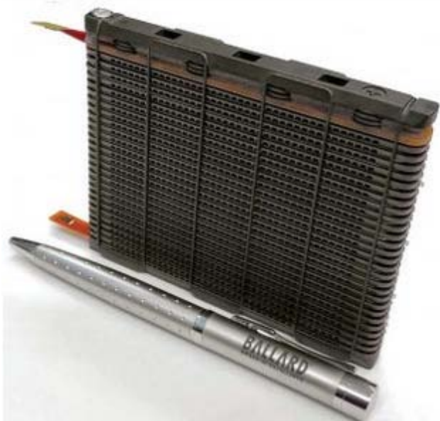
BNPMC-based proton exchange membrane (PEM) fuel cell.
