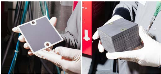
Bloom's fuel cells are fused together, then loaded into metal casings that are enclosed in banks about the size of a refrigerator. Credit Peter Prato for The New York Times
